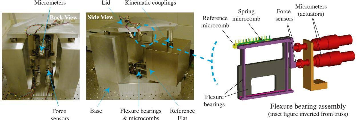
Figure 1: X-ray foil optic assembly truss. *Inset*: Flexure bearing assembly.
