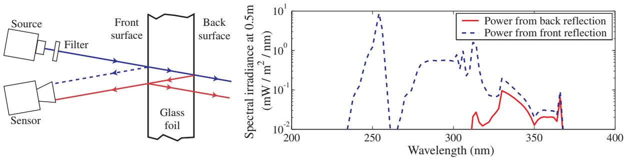
Figure 3: Irradiance from the glass sheets into wavefront sensor as a function of wavelength.
