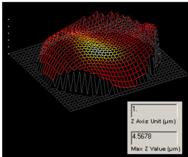
Figure 4: Reconstructed wavefront equivalent to a surface map at the object plane.
