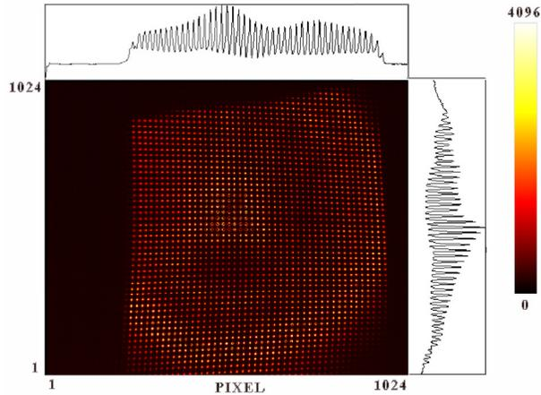
Figure 5: Raw data onto wavefront sensor from Schott D-263 glass sheet.
