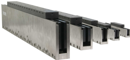
FIGURE 2. This photo shows of a typical family of U-channel (ironless) linear motors. The largest size has a cross section of approximately 50 mm x 150 mm. The magnetic field is largely confined to the track, and the tracks are stacked as needed for the required travel.
