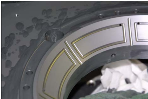
FIGURE 10. Spherical surface after lapping.
