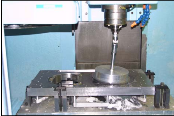
FIGURE 9. A CNC machining center, driving through a universal joint, spins the spherical lap on an axis that orbits using circular interpolation.
