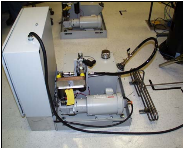
FIGURE 4. Hydraulic power units for the C-axis (far) and the X, Z and B axes (near).
