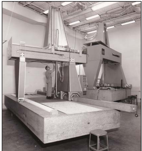
First extremely large air bearing CMMs. Electro Motive (foreground) and Y12 (background)
