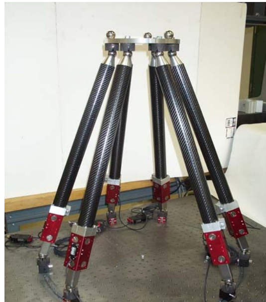
Figure 1 6-DOF Measuring Device [Zhu and Cui, 2001, patent pending]
