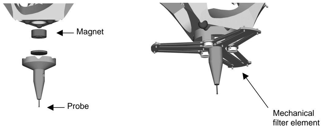
Figure 4: Magnetic holding of the probing element (left) and mechanical filter (right).
