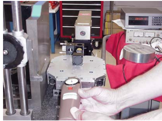
FIGURE 10. Mapping shear stiffness with laser interferometer and force gage.
