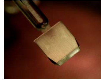
Figure 8: Molded plastic precision blade.
