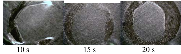
Figure 10 Pictures of welds at various heating times
