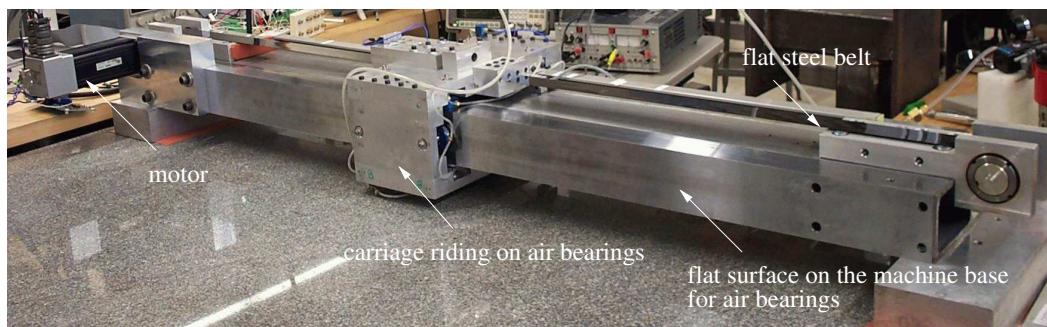
Figure 1. Photograph of the belt drive showing the machine base, carriage, motor, belt, and pulleys
