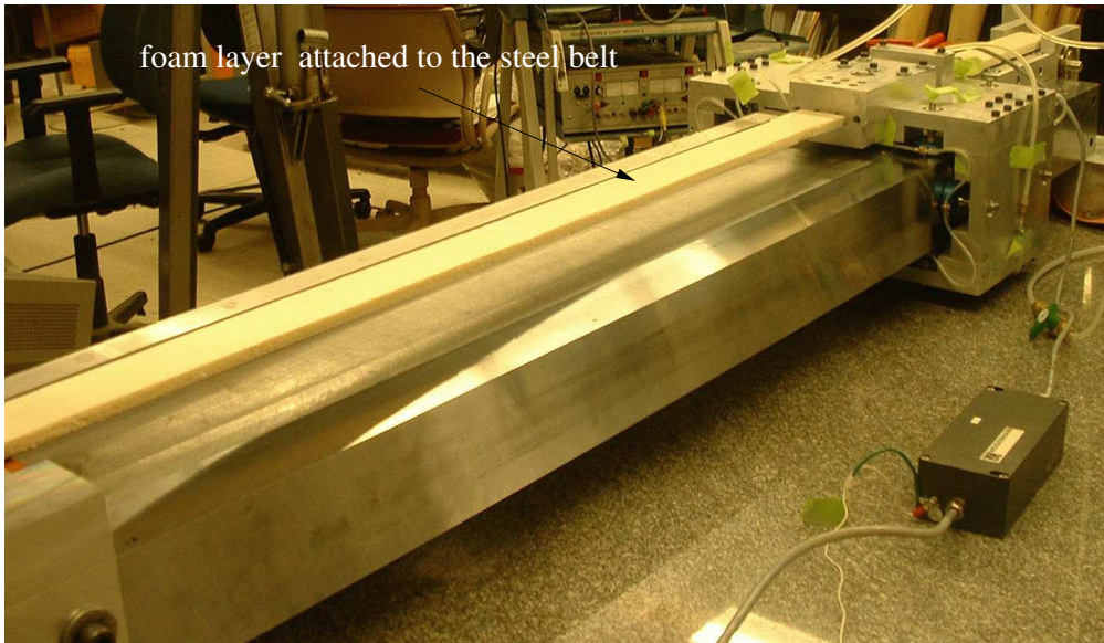
Figure 5. Photograph of the belt drive with 12.7 mm C3201 EAR 10 foam attached to the belt
