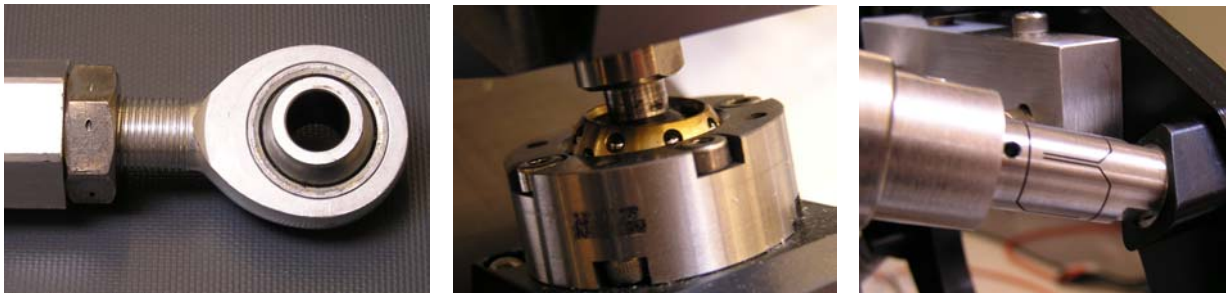
Figure 6: Three of many possible kinds of strut ends
