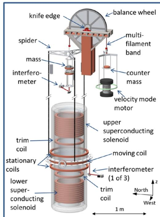
Figure 1 Schematic drawing of the NIST-3 watt balance.
