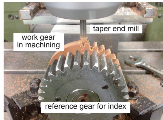
FIGURE 2. The situation of the machining test of this new gear cutting.
