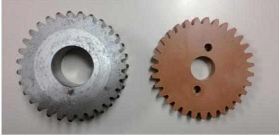
*FIGURE 3. The left one is produced by the hobbing machine for the reference and the right one is the machined gear by new method.*
