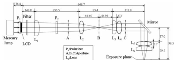
Fig. 3. Optical configuration of the LCD lithography experimental system.
