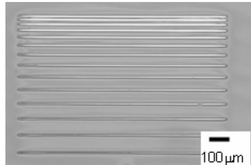
Fig. 5 Line pattern with a width of 10.8  $\mu\text{m}$  width at 12.9  $\text{mJ}/\text{cm}^2$  light as a light source, was useful for 2D device fabrication.
