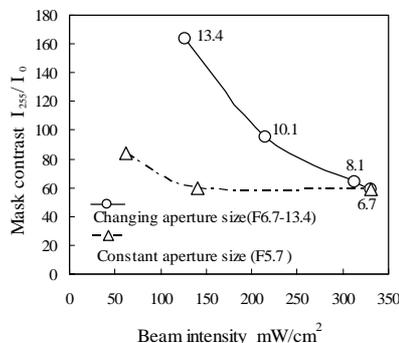
Fig. 2 Influence of light intensity on LCD mask contrast as a function of F-number.
