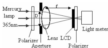
Fig. 1 Experimental setup for characterization of LCD mask contrast.
