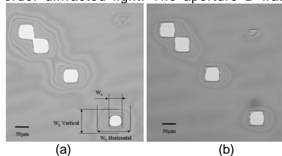
Fig. 4. Typical positive photoresist patterns formed by using LCD mask with LCD lithography system: (a) Exposed at exposure energy of  $66 \text{ mJ/cm}^2$  ( $0.168 \text{ mW/cm}^2 \times 390 \text{ s}$ ) without any aperture; (b) exposed at exposure energy of  $15 \text{ mJ/cm}^2$  ( $0.025 \text{ mW/cm}^2 \times 600 \text{ s}$ ) with 8mm-diameter aperture C.
