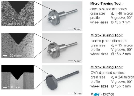
FIGURE 1: Micro-diamond tools for truing CBN micro-grinding wheels.
