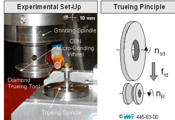
FIGURE 3: Trueing of a CBN micro-grinding wheel by an electro-plated diamond trueing tool with grain size of 46 micron
