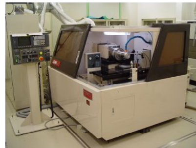
FIGURE 3. Single-point diamond turning machine in a temperature controlled clean room.
