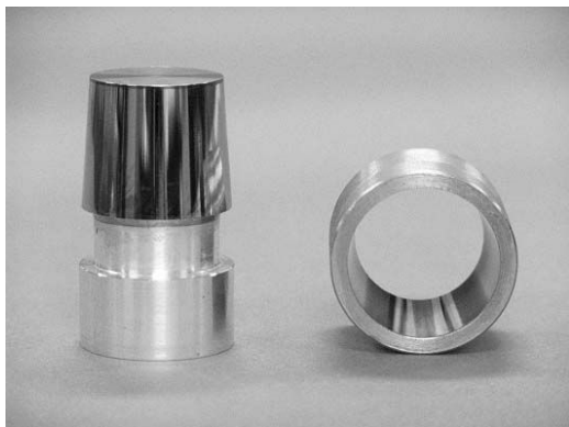
FIGURE 6. Diamond turned and polished conical electroless nickel mandrel (left) and replicated Pt/C multilayer conical mirror (Right).
