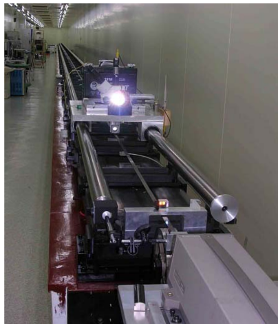
Figure 1: Overview of the 50 m tape measuring system.
