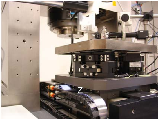
FIGURE 3. Close-up of the linear air bearing stage and one of the pitch/roll/z adjust stages
