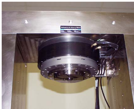
FIGURE 2. Inverted air bearing rotary stage with disc vacuum chuck
