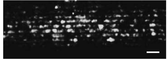
FIGURE 2: Light scattering of interference fringes by \phi 80\text{nm} gold particles (BBInternational Ltd. EM.GC80). A total of 100 consecutive frames were integrated at an exposure rate of 30ms/frame. Scale: 10 \mu\text{m} .
