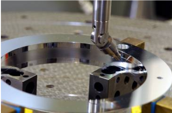
FIGURE 5. Setup of a CMM probe measurement of the swept sine waves.
