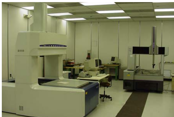
FIGURE 1. The Legex CMM (on left) in the Plymouth Calibration Laboratory of Mitutoyo America.
