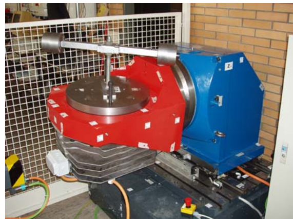
FIGURE 2. Exemplary machine tool manipulator with 3 direct driven DOF [1]
