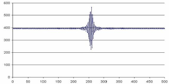
*FIGURE 1 : Interference signal corresponding to the mean of 16 locations for the triplet thin-film coating. The interference objective was a x10 Mirau (0.3NA) and the pixel-binning was 2\*2. The surface area of the 16 locations was (10µm)<sup>2</sup>*
