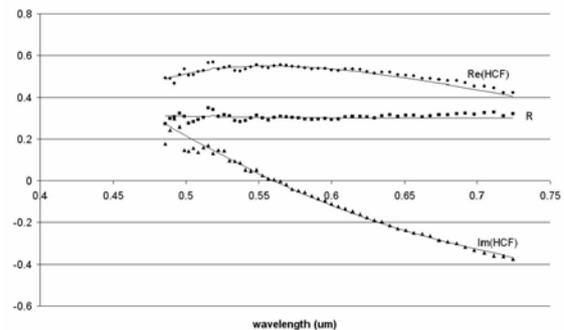
FIGURE 5 : Extracted and fitted HCF function (real and imaginary components) and spectral reflectance,  $R(\nu) (= |HCF(\nu)|^2)$  for sample A..
