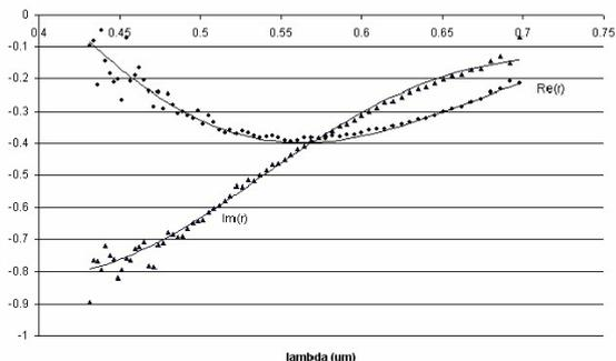
FIGURE 3 : Electrical Field reflectance for the triplet thin-film coating in terms of real and imaginary components. Also shown in solid lines are the corresponding components derived from the thin-film optimisation.
