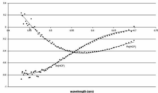
FIGURE 2 : HCF (Helical Conjugate Field) function corresponding to the triplet thin film sample. The real and imaginary components are shown. The solid lines are the corresponding real and imaginary components obtained through thin-film optimisation.
