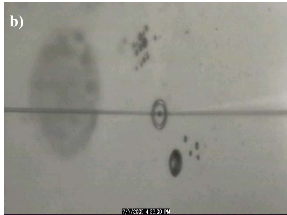
Fig. 6: a) Illustrates the set-up for fill-tube insertion into the counterbore. b) Glass fill-tube inserted and adhered to a 12 \mu\text{m} diameter, 10 \mu\text{m} deep counterbore in an aluminum test sample.
