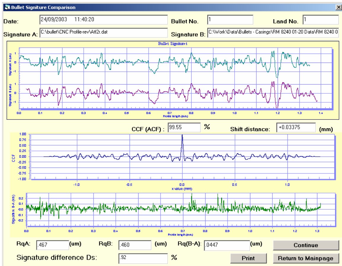
Fig. 1. User screen for a bullet profile signature comparison of S/N SRM 2460- 001 standard bullet (Signature B, shown as the second profile from the top) and the virtual standard (Signature A, shown on the top). The maximum of the cross-correlation function CCF_{max} = 99.55 \% , the signature difference D_s = 0.92 \% . The units of the top and bottom vertical scales are \mu\text{m} . The units of the lateral scales are mm.
