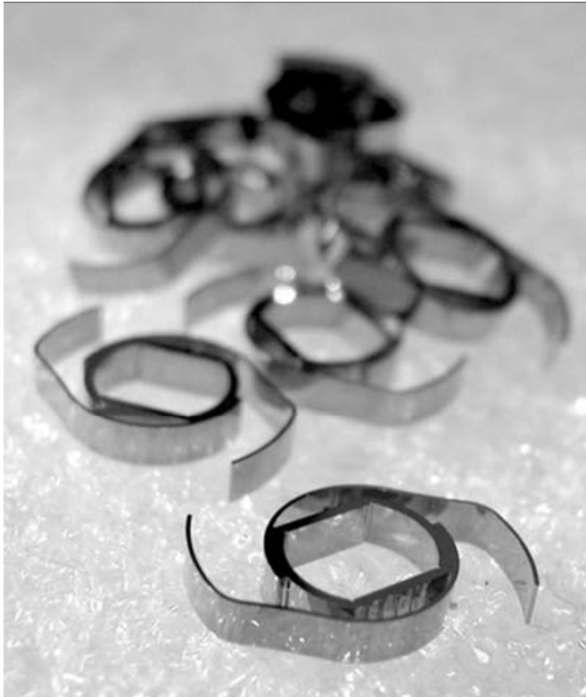
Figure 1. LIGA fabricated part for inspection by video system. This part is typically 10 mm wide by 1.5 mm tall. (From ref. [1]).
