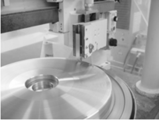
Fig. 1. Single point diamond turning of a tin lap.
