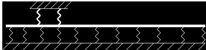
Figure 2: FE Model of the tool air-bearing and friction wheel
