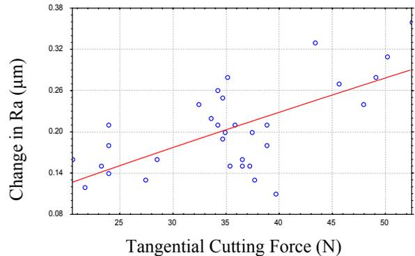
Fig.5b Correlation between Tangential Cutting Force and Change in Ra
