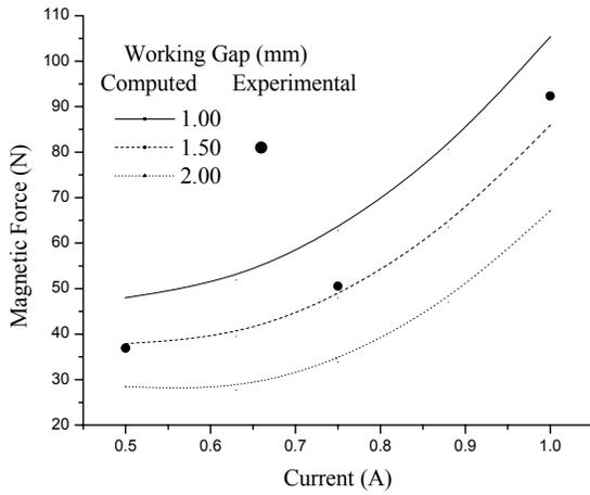
Fig.3 Effect of current on magnetic force for different gap at %oil = 3, RPM = 125, Time = 45min
