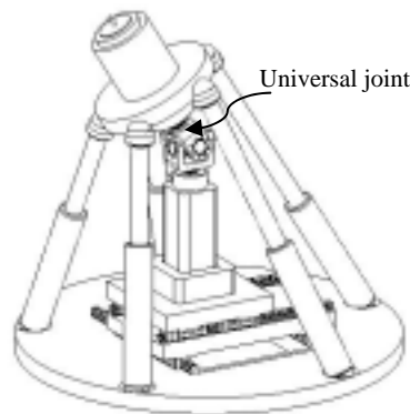
Fig.3: The architecture of the Cartesian guided Pentapod
