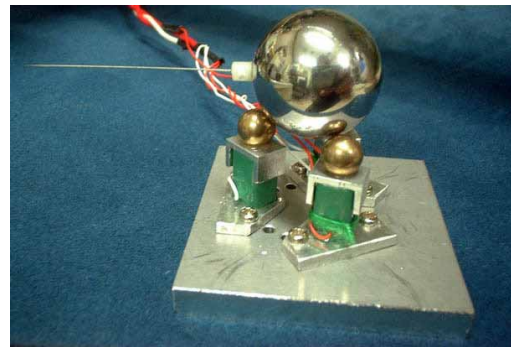
Fig.7 Spherical micro manipulator provided for microscopic manipulator
