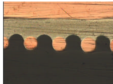
Figure 8. Axial cross section of the micro screw
