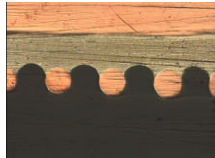
Figure 8. Axial cross section of the micro screw
