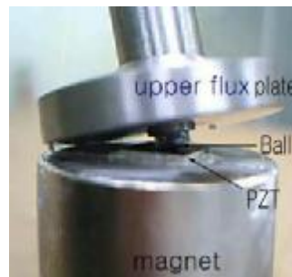
Fig. 4 Ball joint with φ 2 mm ball
