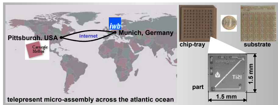
Fig. 3 Transatlantic tele-operated micro-assembly: experimental setup
