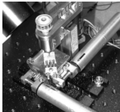
Fig. 6 Prototyped miniature mill (type 12036)
