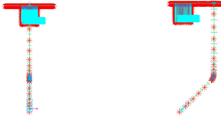
Figure 2: Finite Element model of Feedback spring assembly.
