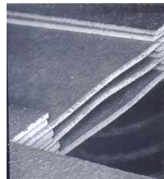
Figure 2. SEM micrographs of a microchannel heat exchanger with nonuniform flow channels after fin buckling
