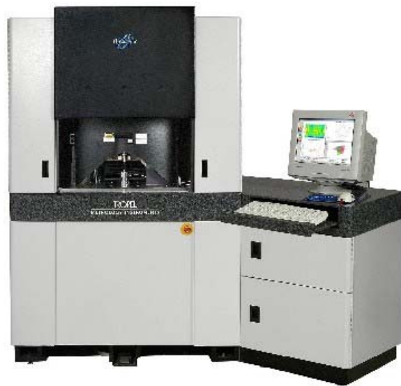
Figure 1. The new machine can measure rough cylindrical and conical surfaces inside of blind holes.
