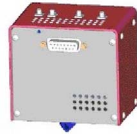
Figure 2. The sensor head contains the DFB laser, optics, detectors, and electronics.
