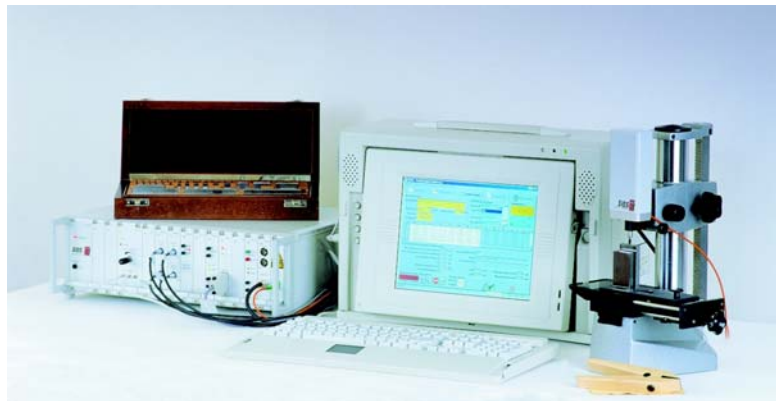
Fig. 3: View of a gauge-block calibration system equipped with a laser-interferometric gauging probe.
