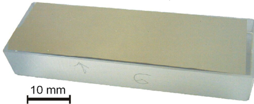
figure 1: 10 nm Pt-film on a fused silica substrate as thickness standard for X-ray facilities
