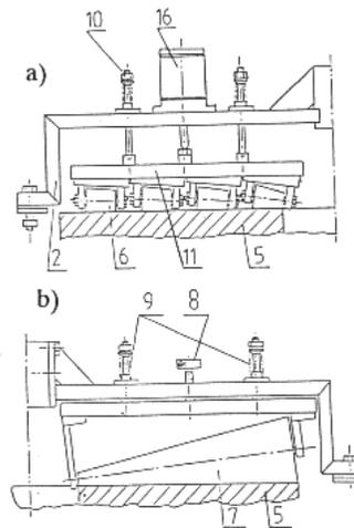
Fig.2. Conical roller assembly for lapping tool charging (a) and the position of the abrasive micrograin distributing rubber roller (b)
