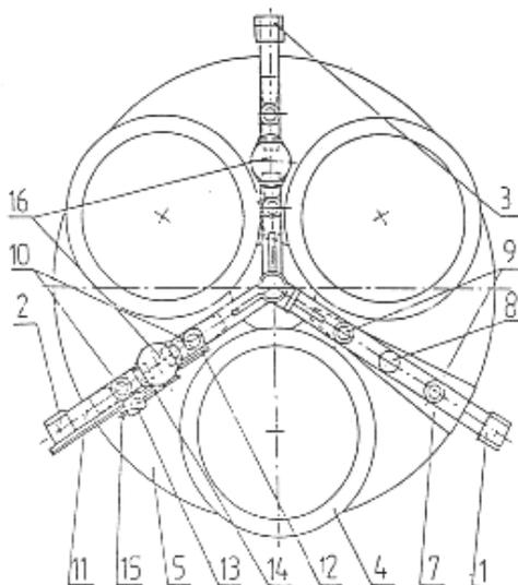
Fig.1. General top view of the productive version of the device for abrasive charging of the lapping tool surface
