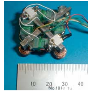
Fig.8 Versatile micro robot provided for microscopic operation
