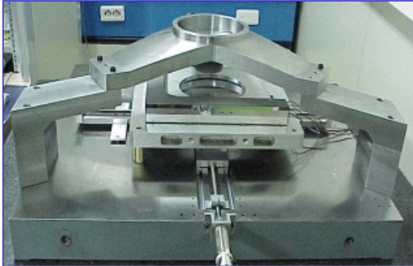
Fig. 5 prototype nano-measuring machine under developing.
