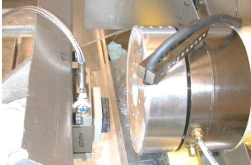
Figure 1: Close up view of air bearing spindle with flycutter head, dynamometer, and silicon workpiece. A hose for coolant is shown above the workpiece/tool contact point.
