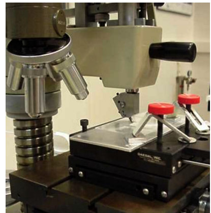
Fig. 3. Setup for scribing tests.
