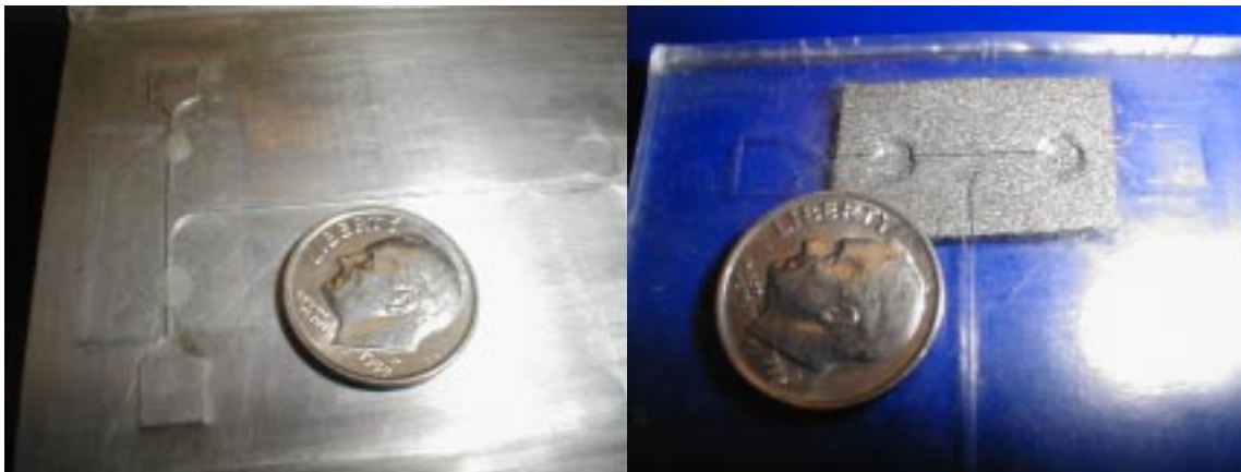
Figure 3. (Left) Master aluminum part, which has raised channels, wells, and dimples. (Right) After replica molding, the elastomer microchannel is peeled from the master. Two magnetic valves are shown.
