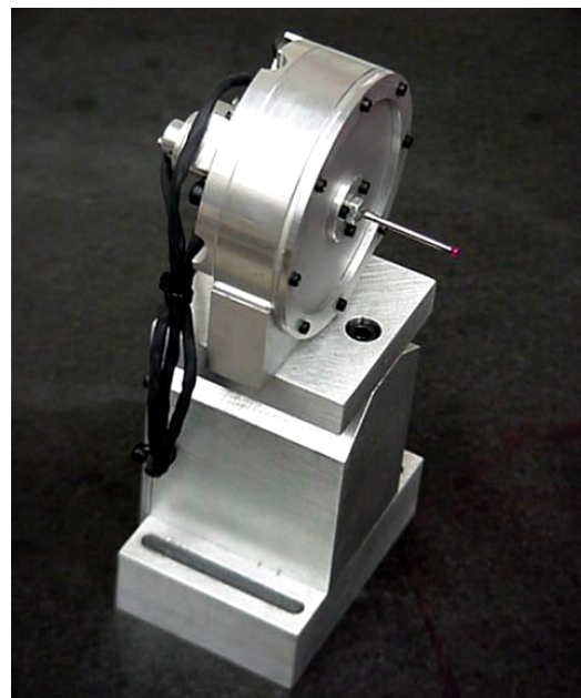
Figure 7. The Three-Axis Measurement Probe mounted on an aluminum stand.
