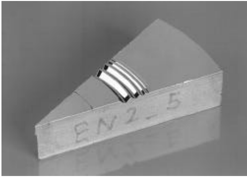
Figure 10: Photo of the new diamond-turned depth setting standard
