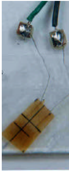
Fig. 3 Photograph of the strain gage mounting on glass surface at 45°
