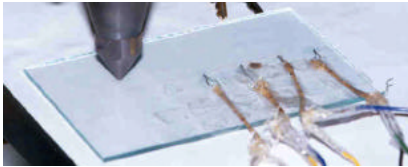
Fig. 2 Thermocouple mountings on plate glass
