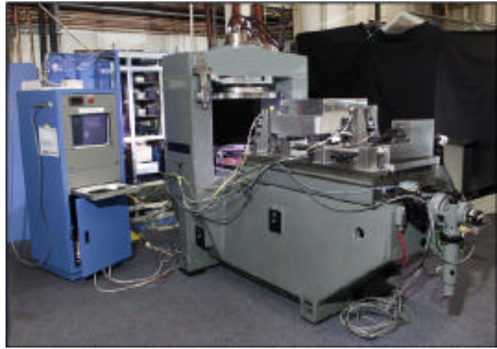
Figure 2: LLNL Prototype Flatness Machine (with workpiece)
